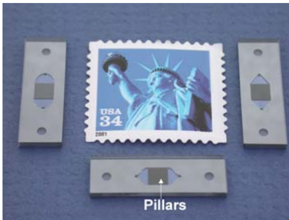
FIGURE 6.2 Arrays of microfabricated pillars with silica surfaces.
