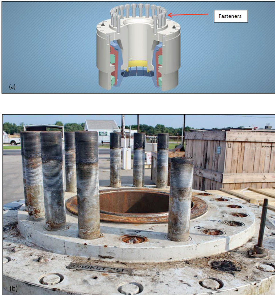
FIGURE 2.3 (a) Sketch of a lower marine riser package (LMRP) connector. (b) Photograph of actual. SOURCE: Bureau of Safety and Environmental Enforcement, Evaluation of Fasteners Failures—Addendum , QC-FIT Report #2016-04, Office of Offshore Regulatory Programs, February 2016, https://www.bsee.gov/sites/bsee.gov/files/qc-fit-nov-bop-bsr-bolt-report-7282017.pdf , pp. 15-16.
