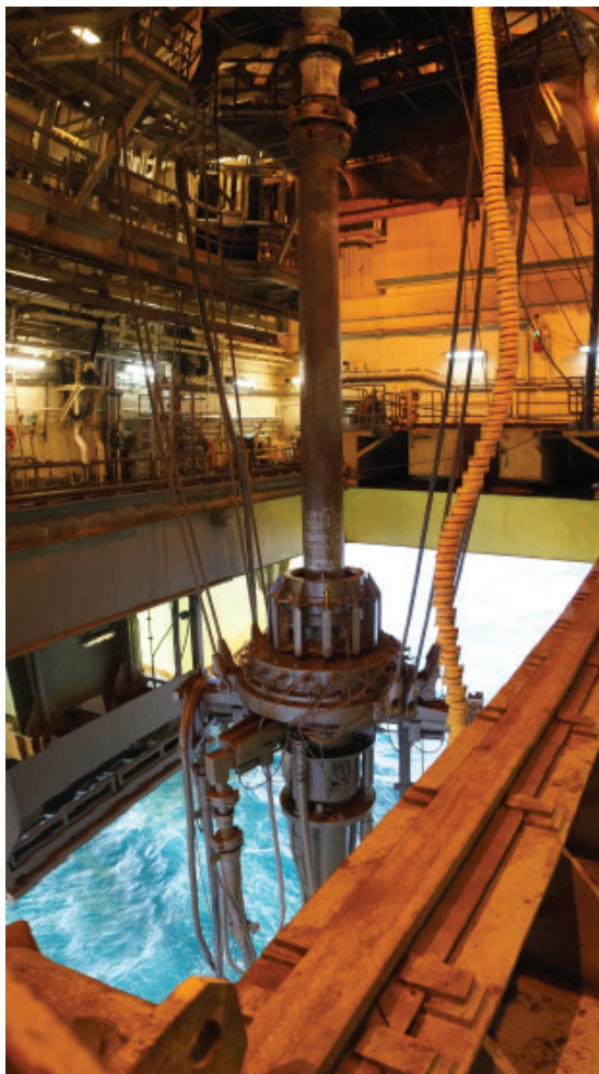
FIGURE I.8 Extended slip joint and riser tensioners in moonpool. SOURCE: iStock Getty Images.
