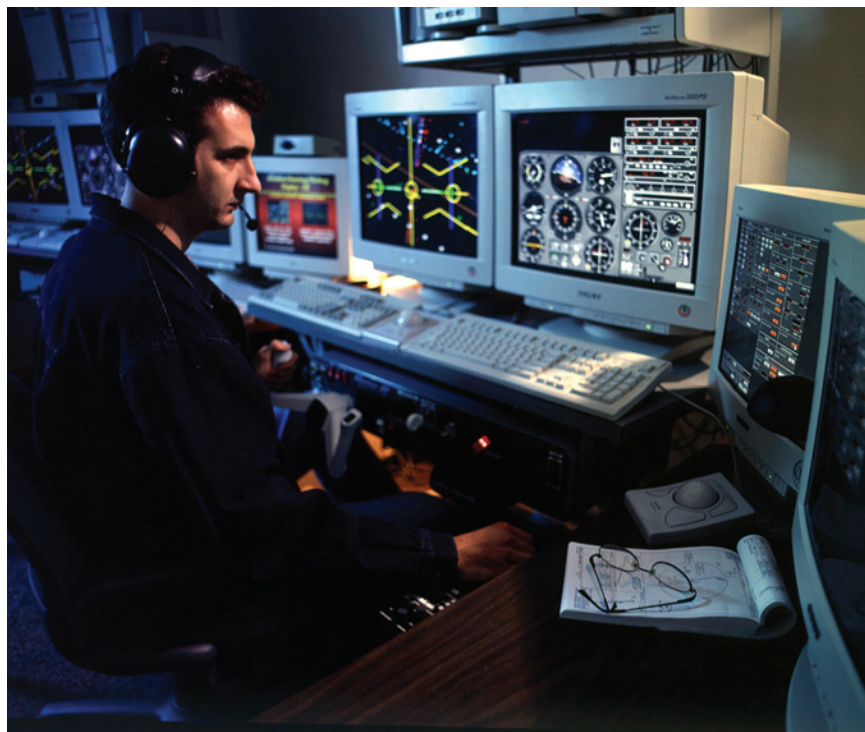
FIGURE 3-2 OZ display (left) versus traditional display (right). Due to the complexity of certification, such flight technologies will probably be applied first for the piloting of UAVs rather than manned aircraft. Intelligence analysts could use displays based on similar principles to allow them to process large amounts of information more reliably. SOURCE: Still and Temme (2001).
