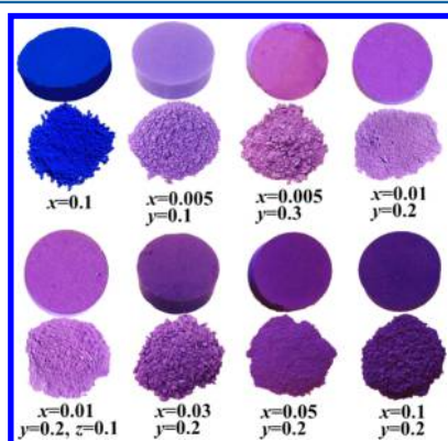
Figure 3. Tuning the color from blue to violet and purple through TBP site substitution. The general formula of the selected compositions is \text{YIn}_{1-x-2y-z}\text{Mn}_x\text{Ti}_y\text{Zn}_z\text{Al}_z\text{O}_3 .
